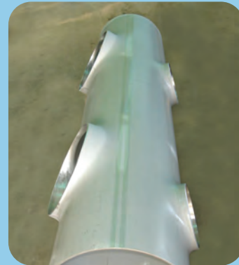
(Figure 6) Different Directions and Diameters of Outlets 不同分歧孔方向與外徑
