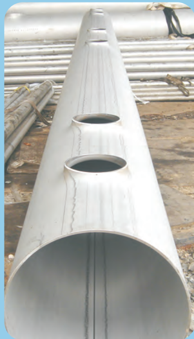
(Figure 2) Branching Outlets 分岐孔
