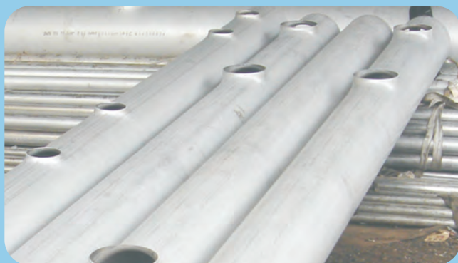
(Figure 3) Branching Outlets 分岐孔
